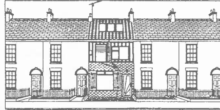
Alterations not requiring consent include doors and windows, shutters, railings and roof tiles
