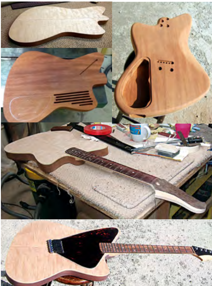
Various stages in the making of an electric guitar, and above right the (almost) finished article
